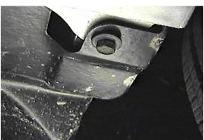
4. Just forward of front tire on the underside of fascia, remove metric bolt with 10MM socket, both sides. Remove one push pin from opening in fascia. Pull fascia forward and set aside.
