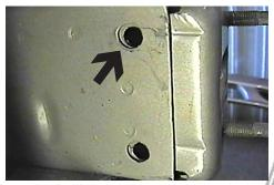
6. Drill out the top existing hole on frame ends with the 13/32" drill bit, both sides.
