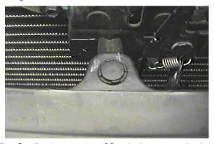
**2.** On the top center of fascia is one push pin to remove.
