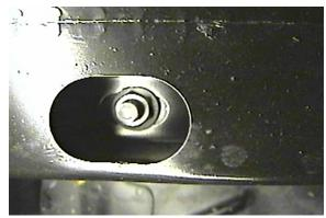
**5.** Remove four metric bolts from metal bumper, pull bumper bracket forward and set aside.
